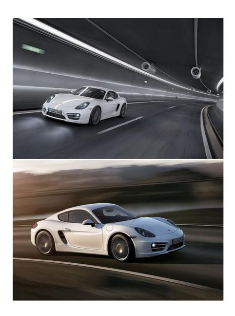
Despite having more power than their forebears, both have in fact had their engine capacities reduced by 0.2 litres. This – along with overall weight reductions, smart energy recuperation systems and a switch to electromechanical steering – equates to economical improvements of around 15% across the range.
