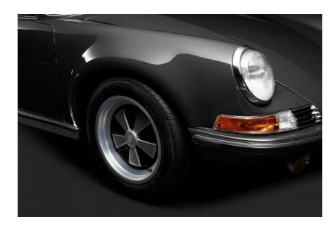
So how do Sadlowski and the PS team create a 911 ST? First of all, they select a 964-series donor vehicle, the penultimate air-cooled 911. This is then totally dismantled and the body fitted with the ST's front bumper and characteristic flared front and rear wheel-arches (an 'RS-style' front spoiler is an option). New indicators, fog lamps and chromed headlamp surrounds are installed. The bonnet is glassfibre – as per the original ST.
