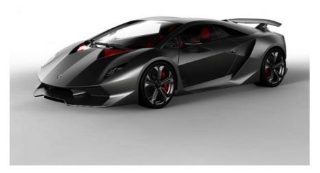
The basis of the car is a solid, stiff, safe and lightweight carbonfibre monocoque cell, while the entire front frame, exterior panels and crash boxes are made from CFRP [carbonfibre reinforced plastic]. The major suspension components and the rims are in carbonfibre, while the tailpipes are made from Pyrosic, an advanced glass-ceramic matrix. Even the propshaft is made of CFRP. The resulting low weight means a car that not only accelerates faster, but also has better handling and braking.
