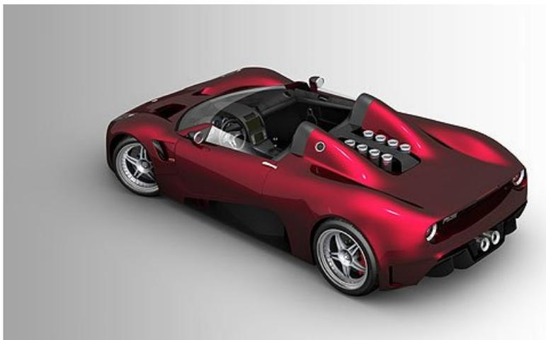
The entire floor pan and external shell is made of carbonfibre, as is the passenger safety cage. The new supercar is powered by a 505hp Chevrolet 8-cylinder engine, embedded in a tubular frame directly behind the driver's cabin.
