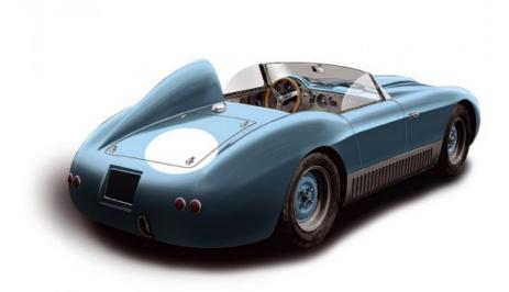
The HB Special uses materials such as aluminium and carbon-fibre which means that the car only weighs 750 kg, its chassis and engine are from the Triumph TR6, improved and re-designed so that the straight-six motor, unlike the original version which had 105 -150 HP, now enjoys over 180 HP. The body is made out of a carbon-fibre shell which is produced in-house in The Netherlands. The cockpit and dashboard are aluminium.
