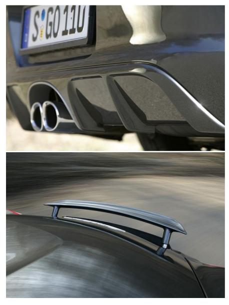
The package includes a front spoiler extension (mounts on standard fitting), an automatically extending, redesigned rear spoiler, and a modified rear undertray with an integrated diffuser.
